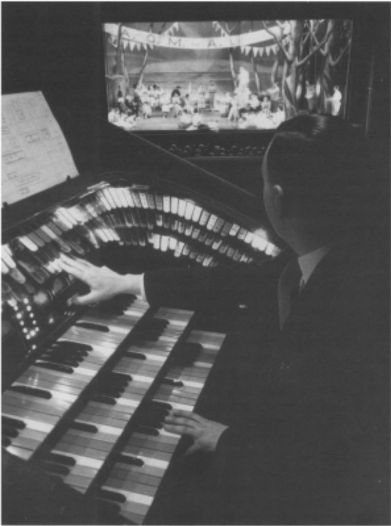
Figure 3.4 The Light Console, modelled on a cinema organ, with a full view of the stage
